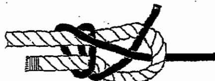
Figure 12-15 The Double Sheet Bend
