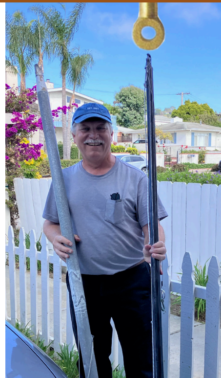
The new spinnaker pole (right) is half the diameter and substantially lighter than the old one (left). An added bonus, it floats!
