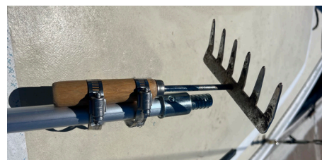
The gardening rake was attached to the extension pole with two hose clamps.
