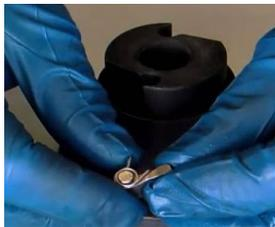
An example of a challenging task is Winch maintenance. The winch is under a lot of pressure to supply leverage and it relies on a surprisingly small part to do it. Replacing worn pawls and springs is a tricky task.
