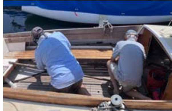
Above: Robert Skillings and Paul Feldon perform surgery on the E1122 woodwork, restoring planks where serious decay had occurred.
