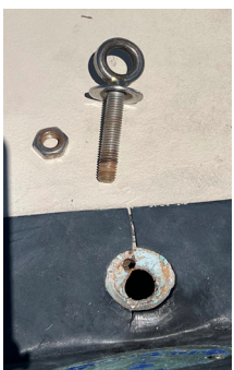
This photo shows the restraining bolt with its matching nut near the hole from which it was coming loose. No lock washers or other washers were attached.
