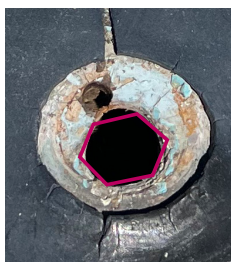
This close-up shows the hole with a super-imposed tracing from the actual nut shown in the photo to the left.
