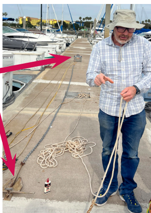
Fleet Captain Tom Bedford replacing the anchor rhode on the E-453. All of the Rhodes were inspected and upgraded (including adding measurement tags to the chains).
