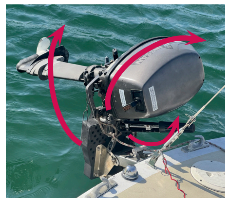
The design of most outboard motors requires they be rotated clockwise to prevent oil leakage.
